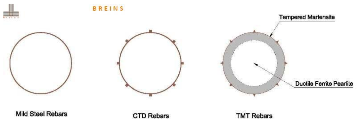
FIG-3, (Cross Sections of Various Steel Rebars Showing their Configuration)
