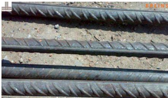
FIG-2, (Longitudinal View of TMT Steel Rebars)
